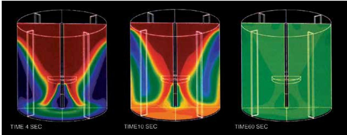
Computational Fluid Mixing (CFM) is a powerful tool that is used to mathematically model fluid flows of different agitator/impeller designs in mixing tanks. Other valuable analyses include the mixing and reaction rates of chemicals and heat transfer. The CFM example above illustrates predicted agitated blend times.
