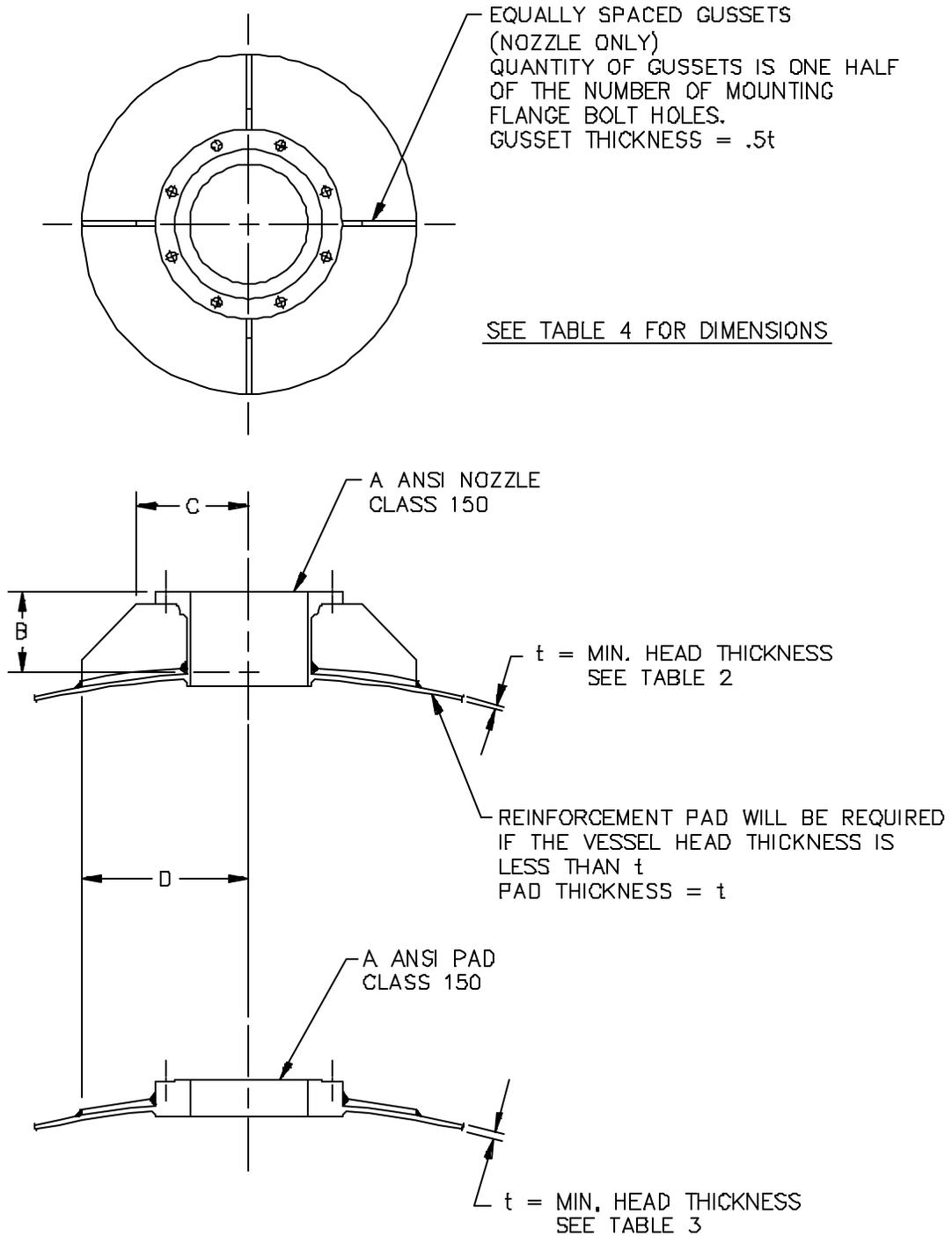
Figure 4: Vessel Mounting Nozzle/Pad
