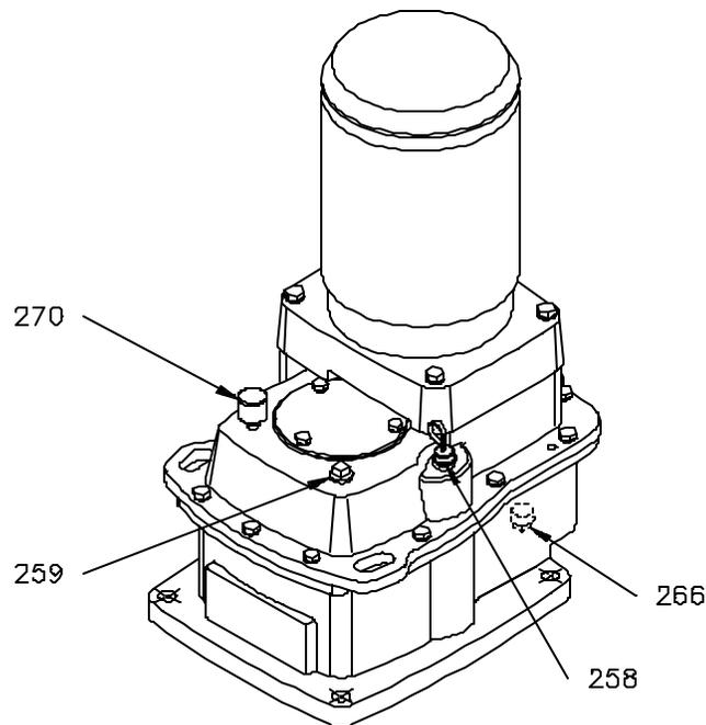
Figure 1: Gear Drive Oil Level Dip Stick
